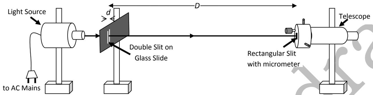
**Figure:** Experimental arrangement to observe just resolved position of the two slits.
