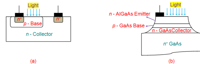
Figure 1 Phototransistor (a) Homojunction Structure (b) Heterojunction Structure
